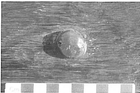
one of the carefully shaped wooden pegs or 'trenails' from the Sizewell boat
