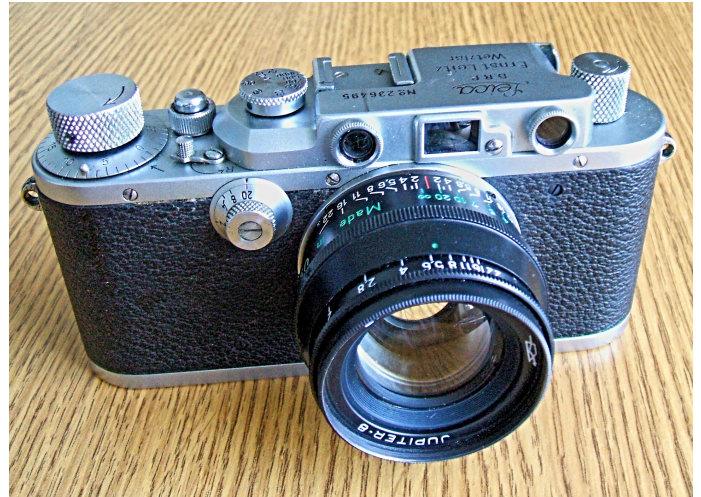
An early Leica similar to the models used by our heroines. Using this, the practitioner can move around selecting up to 36 views before re-loading, though it does have a tripod screw socket on the base for more considered formal records. Note that this particular model has a post-war Russian lens attached! © J Erik Scollay.
