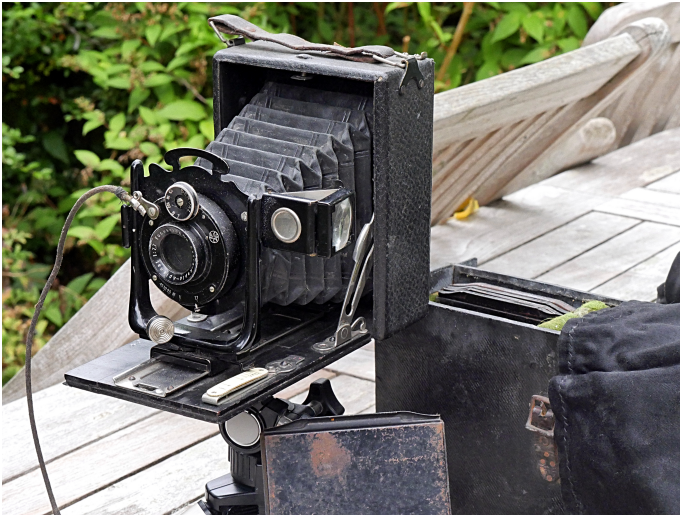
A typical pre-war camera outfit (on a modern mini-tripod). Note the outfit case which holds half a dozen loaded dark slides containing glass plates, a double thickness black focusing cloth, and of course the camera. The camera has a primitive reflective viewfinder attached as an afterthought, but it is clearly intended to be used on a tripod with the black cloth over the photographer's head as he/she attempts to focus the dim, upside-down image on the ground glass screen at the rear. © Eric Houlder LRPS.
