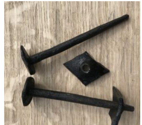
Fig. 5 Some examples of the rivets or iron nails used to secure pairs of planks. © The Sutton Hoo Ship's Company
