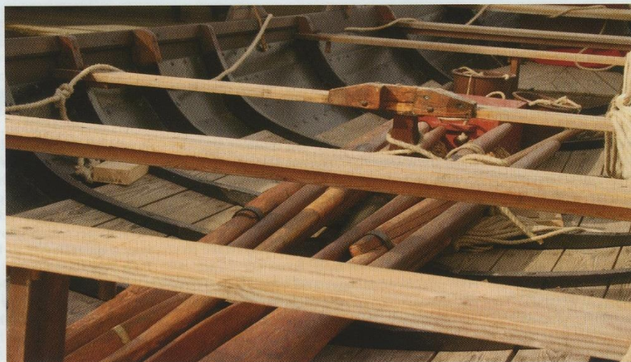
Edwin Gifford added a mast step to his half-scale reconstruction of the Sutton Hoo ship, Sae Wylfing (photo Nigel Maslin).
